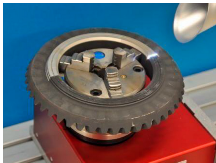
Gear Wheel Rust Cleaning
